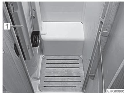
Fig. 157 Pared giratoria grande, girada
