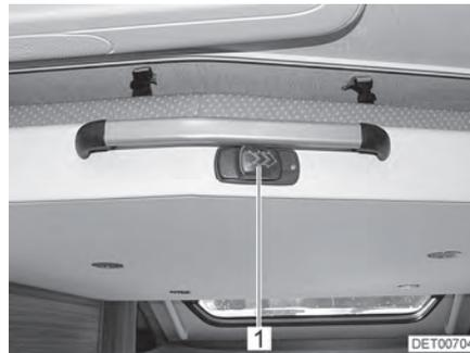
Fig. 75 Pull-down bed with lock
