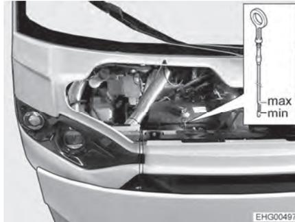
Fig. 12 Oil dipstick (engine oil)
