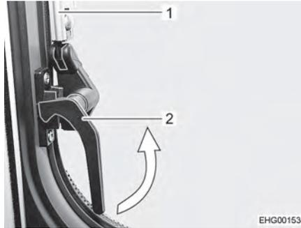
Fig. 39 Catch lever, on the side ("closed" position)
