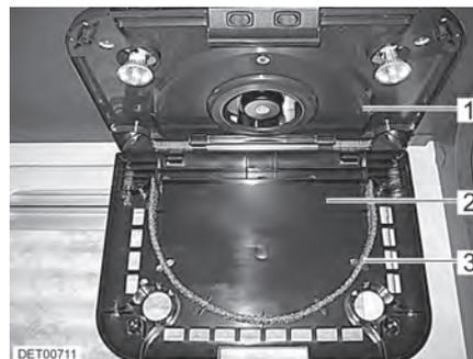
Fig. 160 Removing the grease filter
