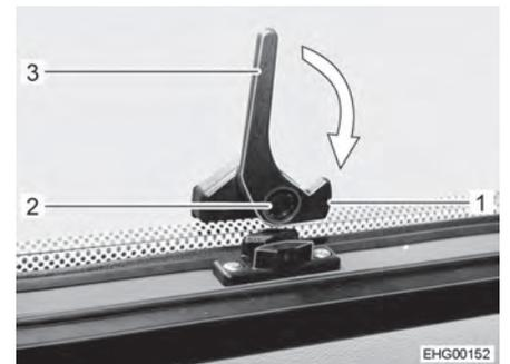
Fig. 42 Catch lever, at the bottom ("open" position)
