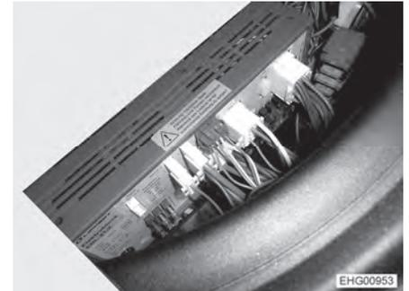
Fig. 99 Transformer/rectifier position (Ford)
