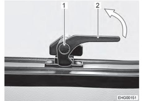
Fig. 40 Catch lever, at the bottom ("closed" position)
