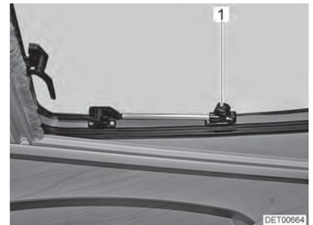
Fig. 47 Roof window with rotary hinges, open
