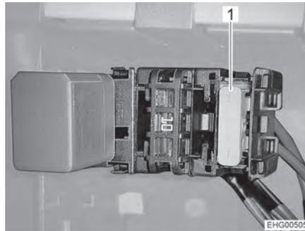
Fig. 113 Fuse on B column, right-hand side of vehicle
