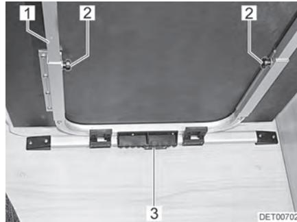
Fig. 58 Shifting/extending the suspension table
