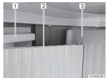
Fig. 151 Correct position of the small swivel wall
