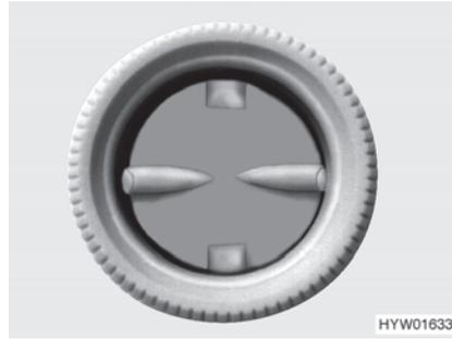
Fig. 119 Air outlet nozzle (hot-air heater)
