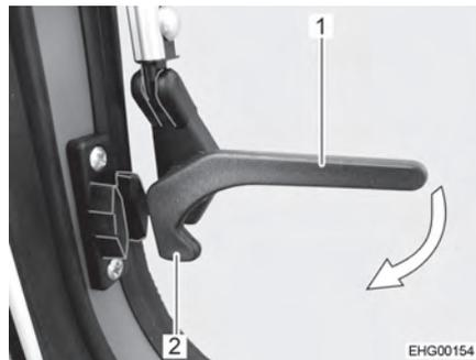
Fig. 41 Catch lever, on the side ("open" position)
