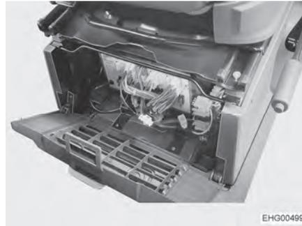
Fig. 98 Transformer/rectifier position (Fiat/Citroën)
