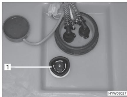
Fig. 140 Water tank with rotary handle
