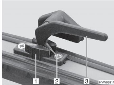
Fig. 48 Catch lever in "continuous ventilation" position
