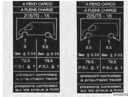
Fig. 173 Tyre pressure information sticker on B column (example)
