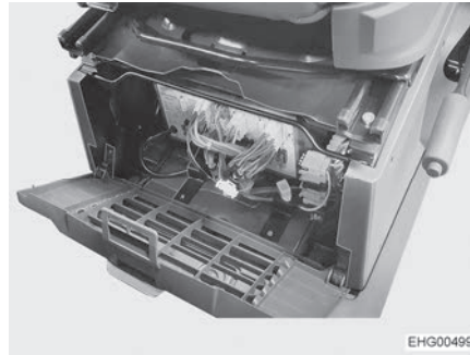
Fig. 97 Transformer/rectifier position (Stellantis)
