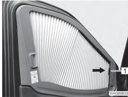
Fig. 26 Side window with folding blind
