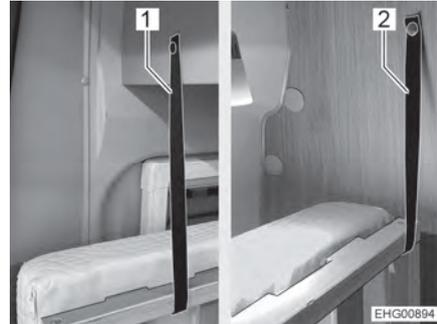
Fig. 47 Retaining straps for left-hand bed
