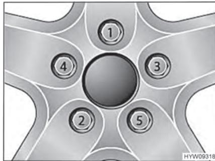
Fig. 127 Tightening the wheel nuts or wheel bolts cross-wise
