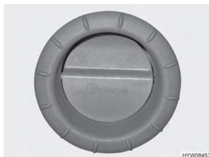
Fig. 92 Air outlet nozzle (hot-air heater)
