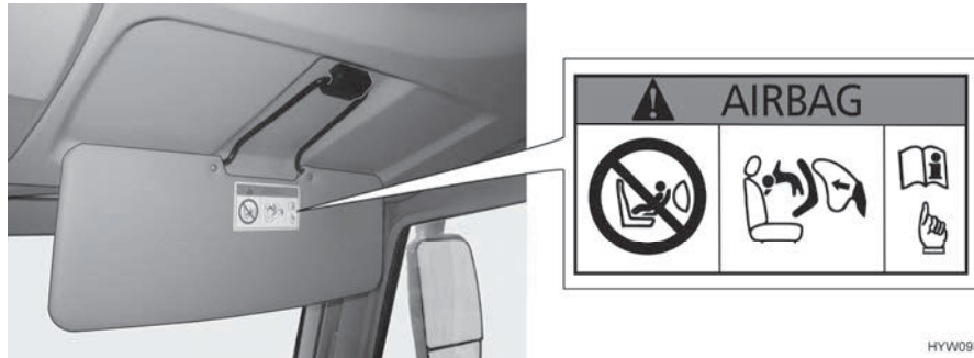
Fig. 11 Warning notice on child restraint system (front passenger's seat sun visor)
