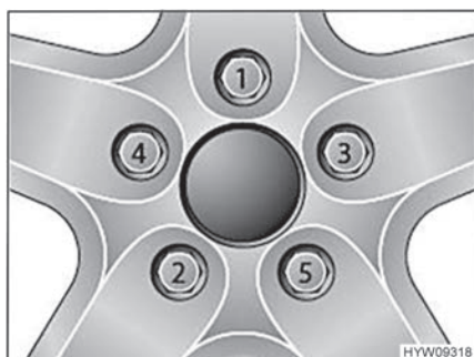
Fig. 130 Tightening the wheel nuts or wheel bolts cross-wise
