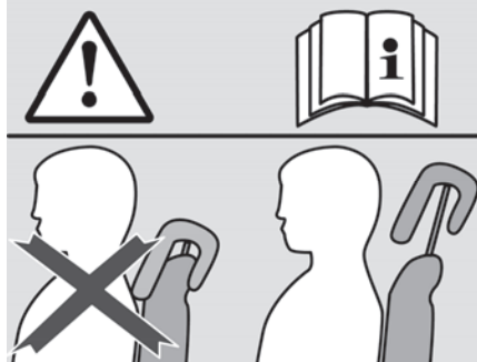
Fig. 16 Correct adjustment of the headrests
