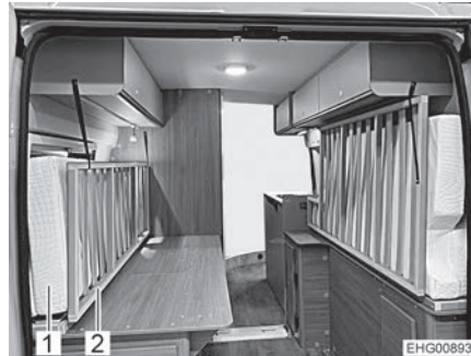
Fig. 47 Mattresses and bed bases transport position
