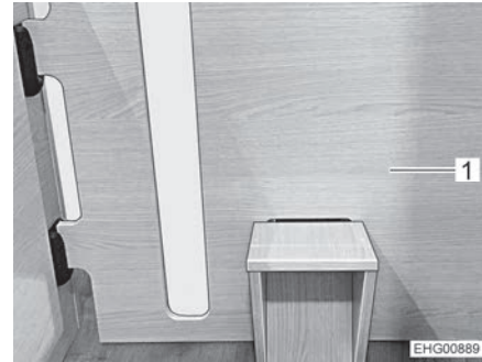
Fig. 43 Partition wall with step unit
