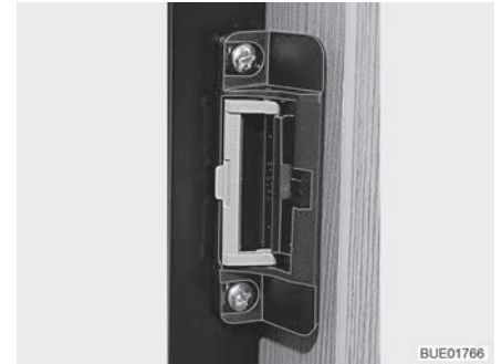
Fig. 104 Locking device in ventilation position
