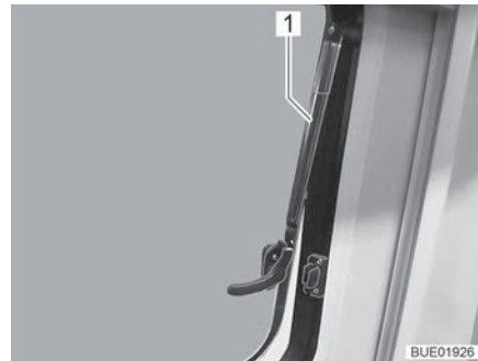
Fig. 20 Hinged window with automatic hinges, open
